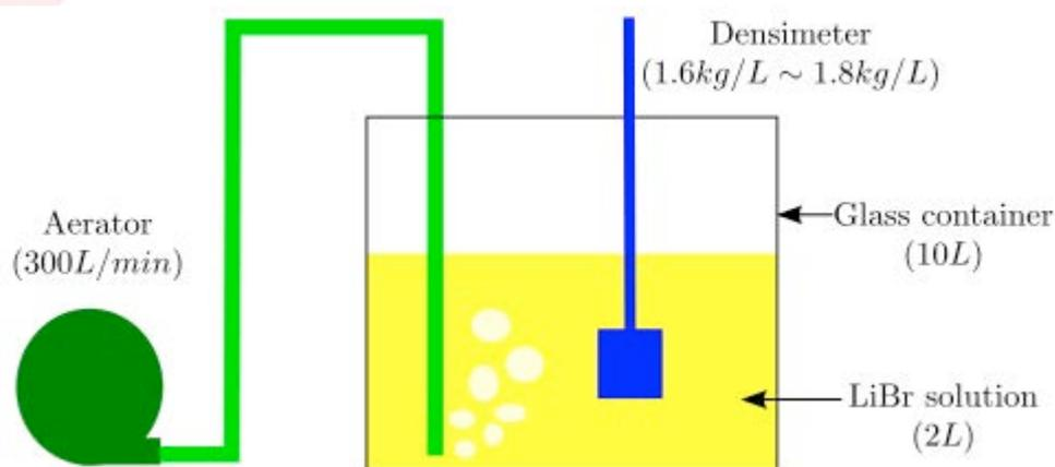
**Fig.4:** Equipment setup of experiments of absorption section
