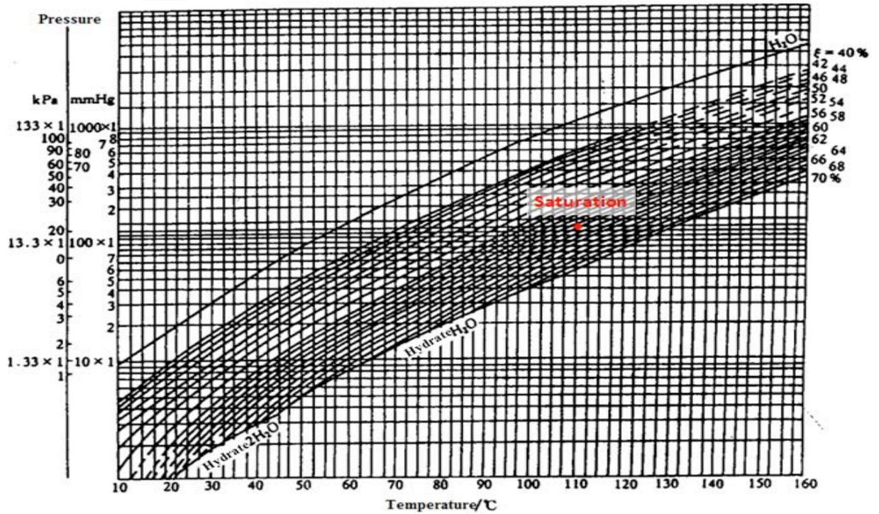
**Fig.1:** Saturated vapor pressure-Temperature-Concentration curve of LiBr solution [9]
