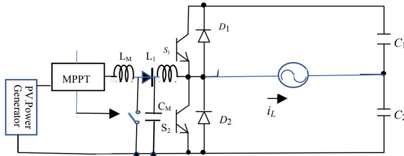
Fig.3. Power Conditioner with Compensation using Boost Converter.
