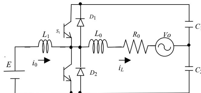
Fig.1. Proposed PCS constructed by half bridge.
