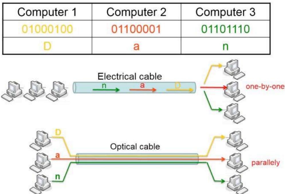
Figure 6: Wavelength Division Multiplexing technique.
